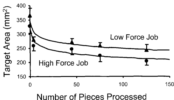
FIGURE 3. Relationship between knife dulling (measured by the carrageenan target area cut) and the number of cuts for the low- and high-force jobs. Average for all employees and plus or minus one standard deviation is indicated. Plots of regression equations in Table I also are included.
