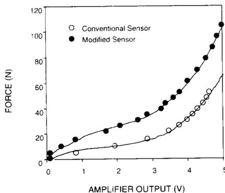
Fig. 2. Representative calibration curves.
