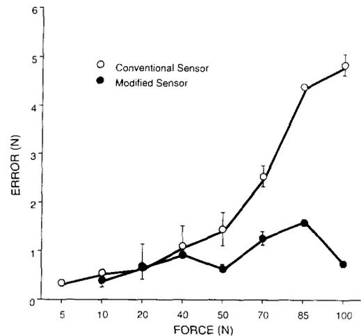
Fig. 4. Average measured error ( $N = 5$  replications) between each sensor configuration and a strain gage load cell.
