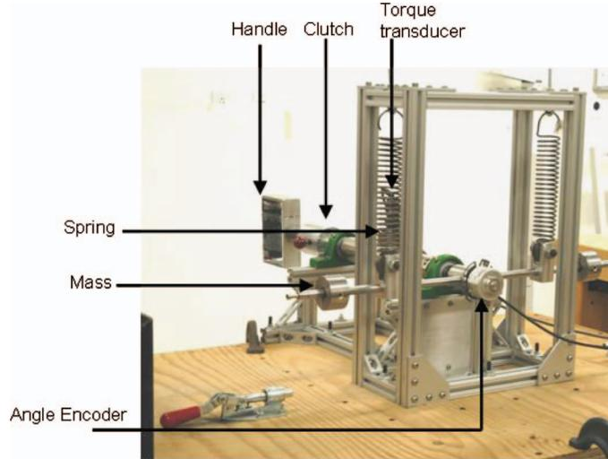
Figure 1. Apparatus for measurement of mechanical properties.
