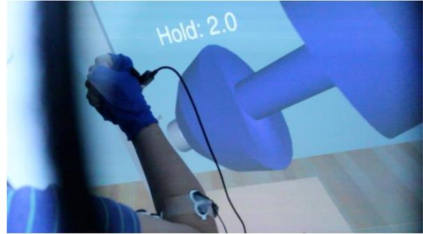
Figure 1. Photograph of a participant lifting a virtual dumbbell in a CAVE (left). An over-the-shoulder view is shown (right). In both photographs the participant observes the dumbbell through binocular vision so it appears to the user as if it is in their own hand. The EMG electrodes are on the arm and an ultrasonic position sensor is attached to a glove on the forearm.
