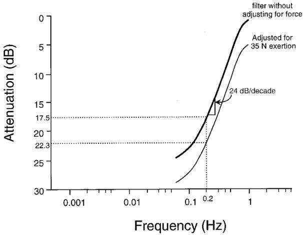
Figure 5. Characteristics of the frequency-weighted filter.
